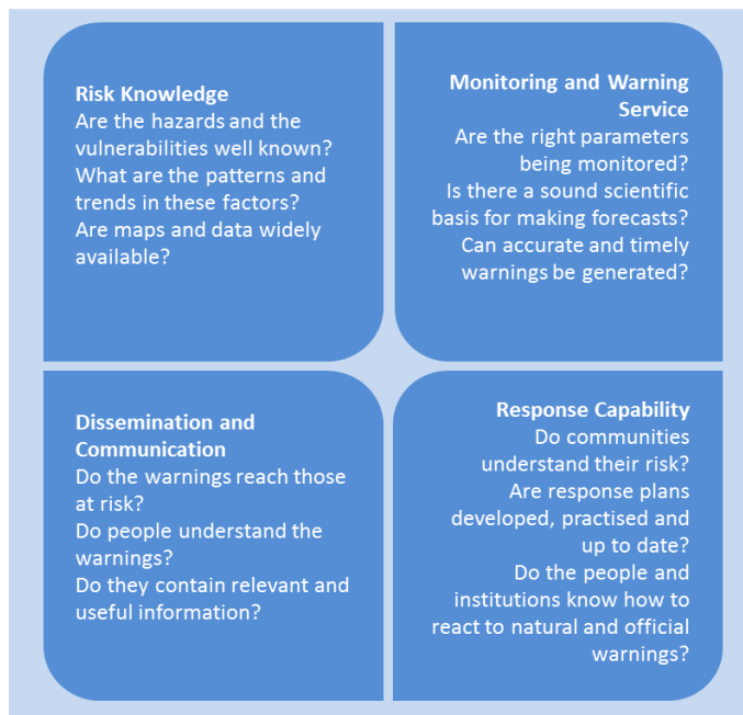
Fig. 2.1 The four elements of a people-centred tsunami early warning system (modified from UNISDR, 2006)
